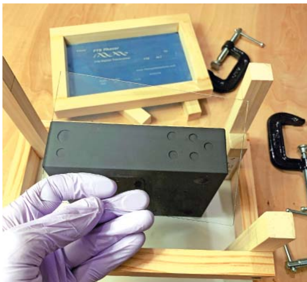
Figure 6 — Using a thin glass spacer between the item you're printing onto and your silkscreen design, will help prevent the ink from smudging.
