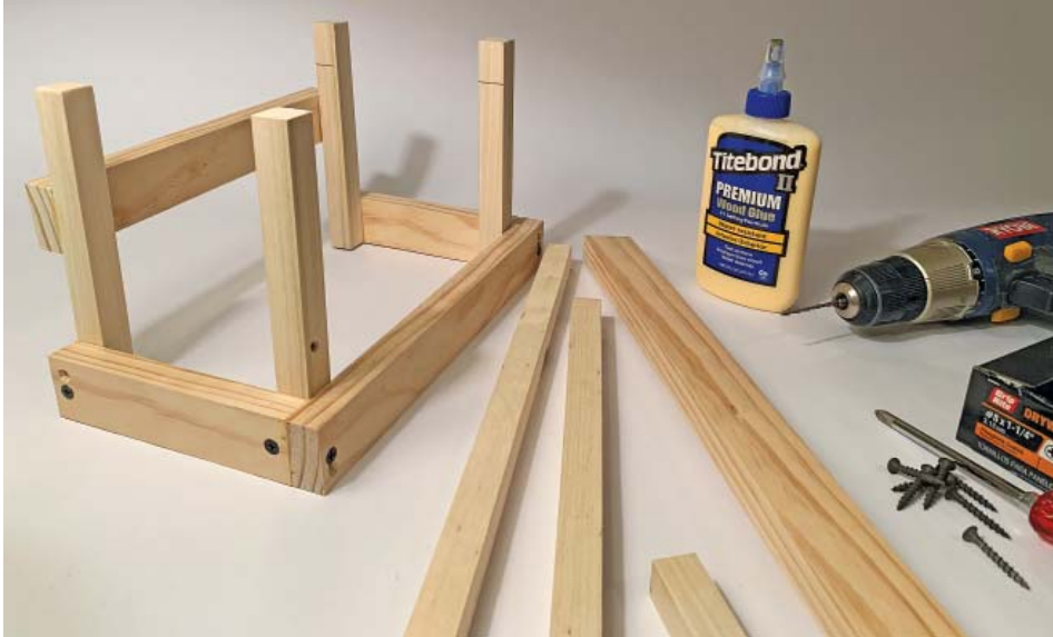
Figure 5 — I needed to build a printing fixture to hold my stencil above my chassis because it was taller than 1 inch. I did this using wooden dowels, wood glue, and inexpensive drywall screws.
