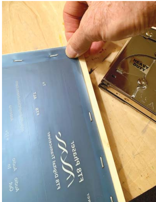
Figure 4 — Hold your stencil tight and flat to mount it to your frame, and secure it using construction staples.
