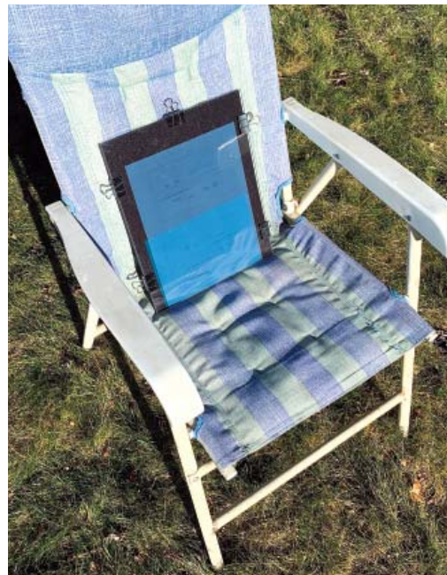
Figure 2 — I exposed my silkscreen design in the sun on a clear day for 6 minutes. Exposure time will vary based on the technique you choose (UV lamp or the sun).
