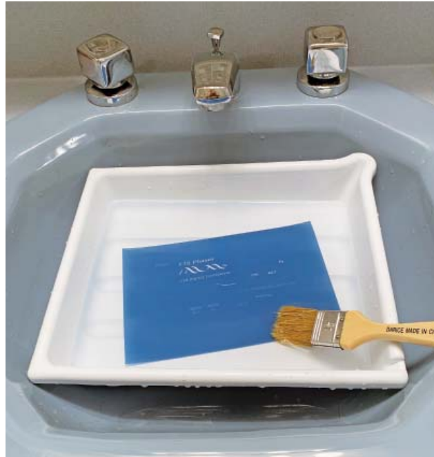
Figure 3 — After your project has been exposed, bring it back to your dimly lit room. Remove the silkscreen from the exposure board unit and submerge it in warm water for 15 minutes. A ghost image of your design should appear.
