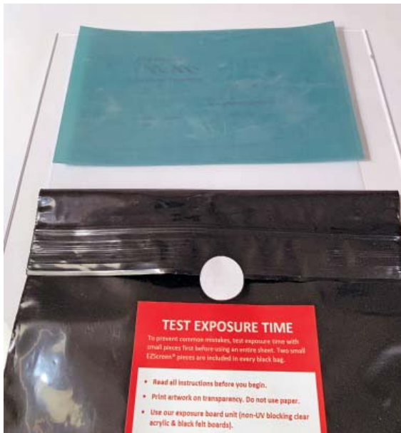
Figure 1 — When preparing your silkscreen for exposure, place the shiny side of your screen face down against your artwork. Your artwork should be facing up, on top of your clear acrylic exposure board unit.
