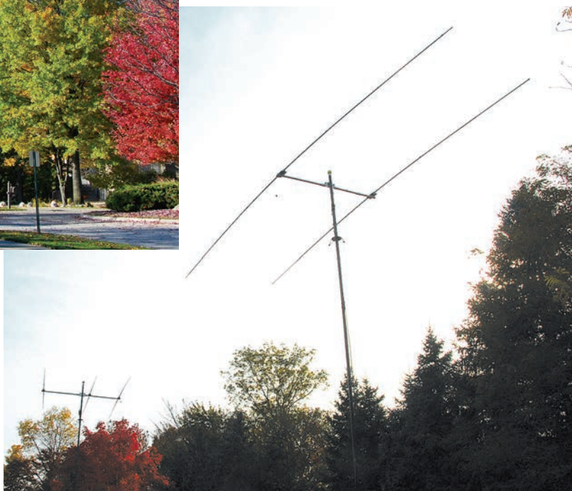
Pete Gladysz’s, K8PGJ, homebrewed three-element 10 meter beam and two-element 15 meter beam, erected just for the W1AW/8 Michigan operation. A full-size 80/40 meter dipole was also put up. Operators were Thaddeus Marlin, W8UE; Mark Shaw, K8ED; Jim Richards, AB8JR; Frederick Czubak, WE8P; David Roberts, KD8RDG; Gerry Treas, K8GT, and Pete, K8PGJ. [Pete Gladysz, K8PGJ, photo]
