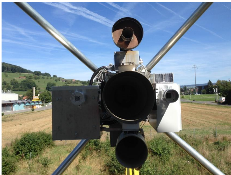
Looking at the business end of the “feed turret” shows how HB9Q puts the big 10-meter diameter dish to work. In the center is the 1296 MHz feed with the 2.3 GHz feed underneath. On top is the 3.4 GHz feed, at the right is the 5.76 GHz feed, and 10 GHz is on the left. (Photo by HB9CRQ)
