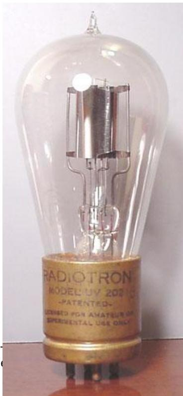
EARLY TRANSMITTER TUBE- RCA UV-202 5 WATT
