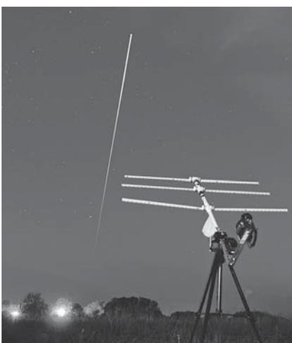
Doug Cook, KD5PDN, made contact with the International Space Station from his back yard in Guthrie, OK, using a homemade antenna made out of an old tape measure. The ISS can be seen leaving a trail in the photo.
