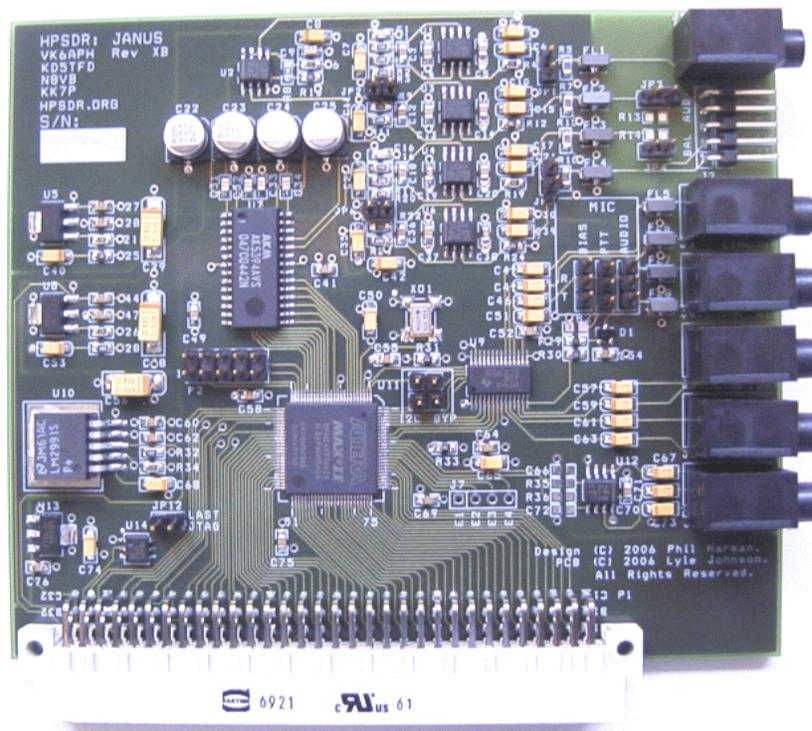
Figure 8: HPSDR's JANUS A/D, D/A module
