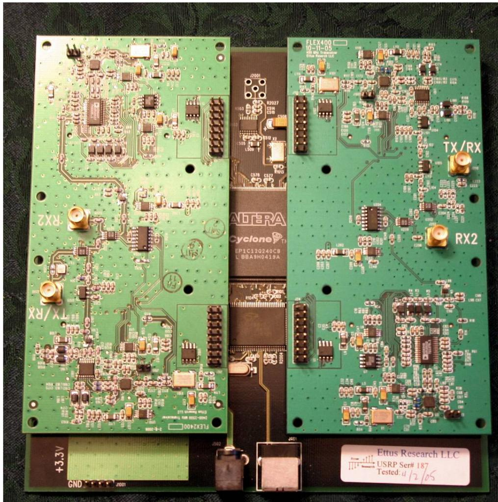
Figure 6: 70cm and 13 cm transceiver modules on the USRP
