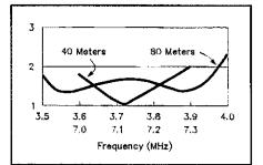
Fig 6—Measured SWR for the 80- and 40meter multiband antenna system.
