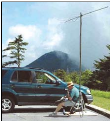
KB5YZG on his first VHF outing (on Mt Mitchell, North Carolina) using an ICOM IC-706, with an 11 element Yagi on top of a stack of fiberglass tent poles. Car battery provided talk power; elbow provided rotator power.
