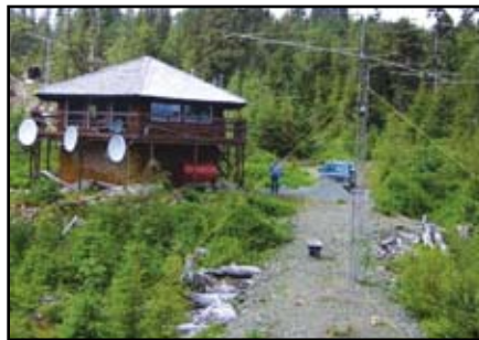
The KL7FF QTH: The 2 meter 12 element Yagi can be seen mounted on the mast on the deck to the left side of the cabin. The 6 meter 8 element Yagi can be seen in the right foreground, mounted on 3 tower sections. The 2 meter station ran 400 W output and the 6 meter station ran 600 W output.
