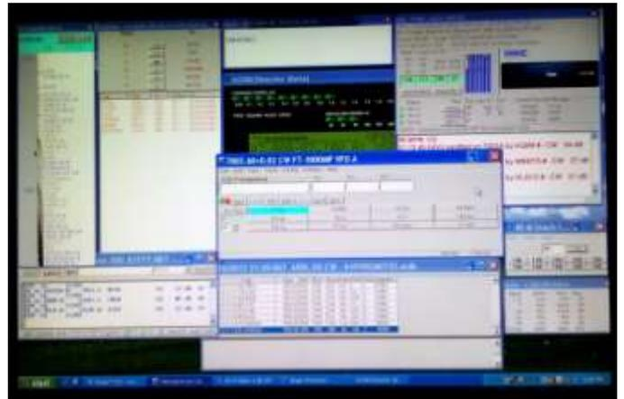
A screen shot taken at K4VV position 1. The operator, N9NC, was running on 40 and, when this photo was taken, had a rate of 164/hr for the last 10 Qs and 111/hr for the last 100. The operator was hundreds of miles away! Operators have complete control of radios, antennas and software from their remote locations. (Photo WØYR)
