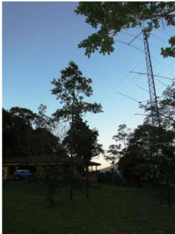
*The TI5W QTH: The 80 foot tower supports an M2 log periodic at the top, 10 and 15 meter stacks and a SteppIR — all bolted to the sides. The tall tree supported one corner of a 160 meter loop. (TI5W Team Photo)*
