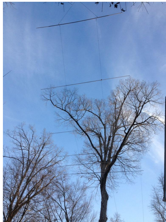
An impressive homebrew 6-element 10 meter antenna by Henry, K4TMC (Photo - K4TMC)
