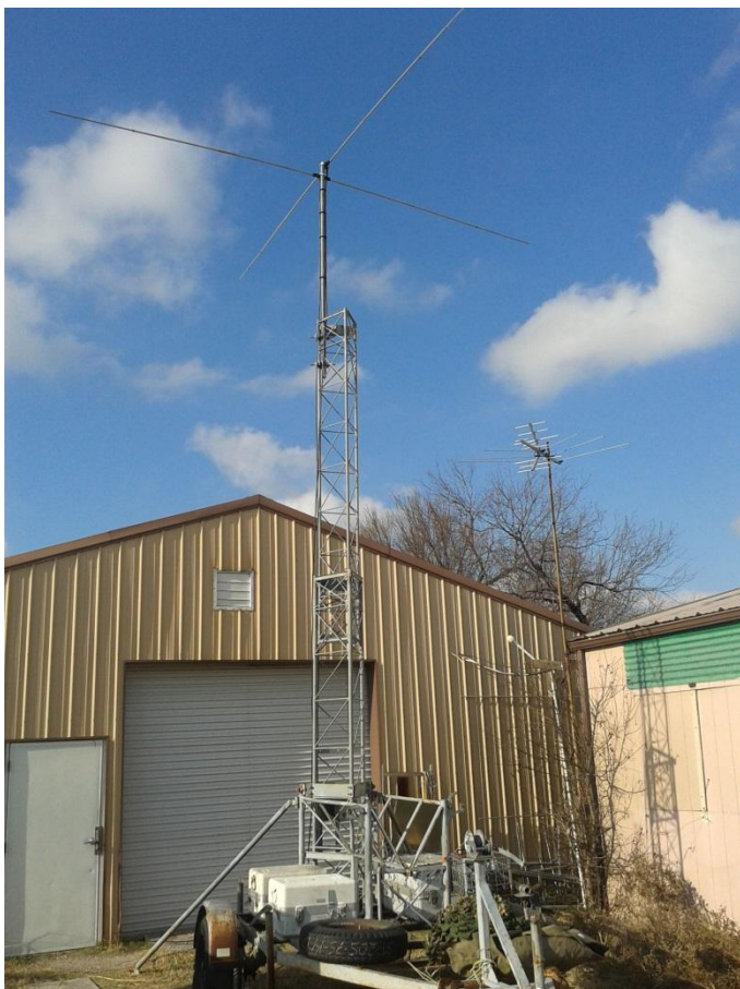
Tim, K7XC's homebrewed crossed dipoles on top of his trailer tower (Photo - K7XC)
