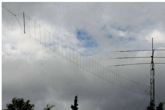
Aimed at the US West Coast, this 50-element, rope-mounted Yagi didn't have a lot of success this year but you can't fault KL7NN for trying! The antenna can be flipped from vertical to horizontal to take advantage of whatever polarization is best. (Photo by KL7NN)
