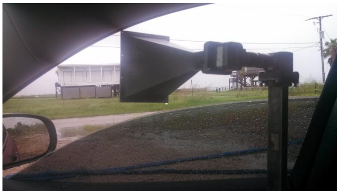
Al, W5LUA operating on the Gulf Coast in the rain. Note the drop of water hanging off the bottom right side of Al's secondary antenna - a horn. This was during two successful 424 km contacts! (Photo credit – Al Ward, W5LAU)
