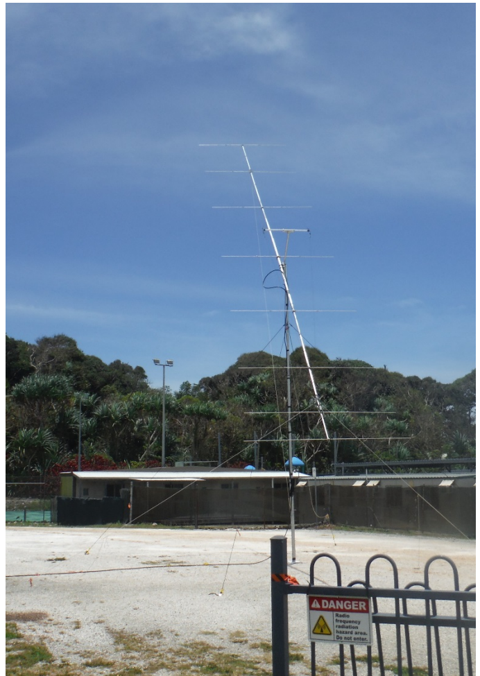
Lance, W7GJ uses this 6M8 Yagi for his DXpeditions. (Photo – credit W7GJ)
