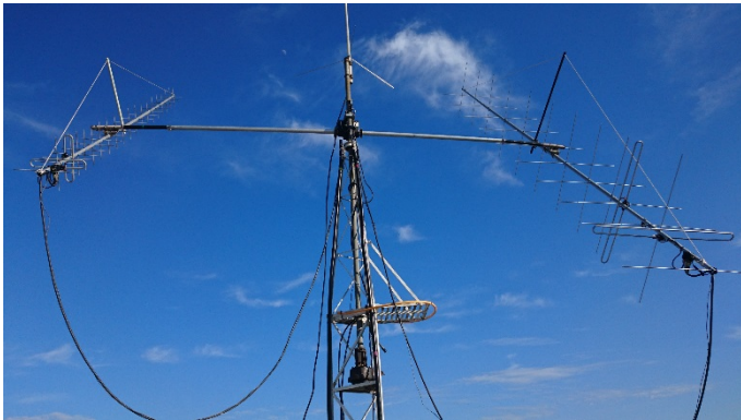
Single cross-polarized Yagis for 2 meters and 70 cm at PY2RN. (Photo – credit PY2RN)
