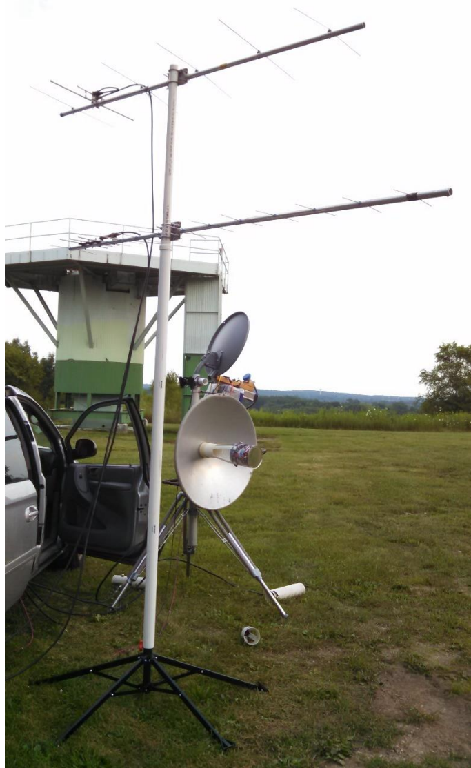
Pete, K9PW is a microwave madman up to 47 GHz! This is his rover antenna setup from the recent 222 and Up Distance Contest (Photo courtesy Pete Walter, K9PW)
