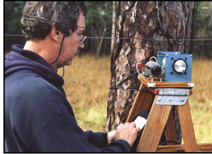
Ray, WA4KEJ, adjusting the inverted L tuning unit at the K4ZM station.
