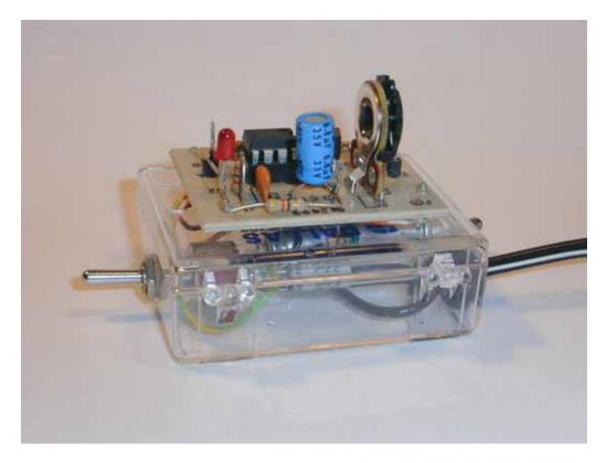
The Ramsey Kit UT-5 Universal Timer makes a handy pulse generator at low cost. It is easily modified to have multiple ranges and an output indicator.
