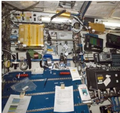
Image of a radiation detector (gold cylinder) and spectrometer (gold box) as part of the DOSIS-DOBIES experiment in the US Lab.
