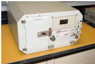
Image of VCKAM cabin air monitor during testing at KSC.
