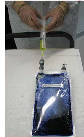
Injection of Osmotic Concentrate into inner partition of FOB.
