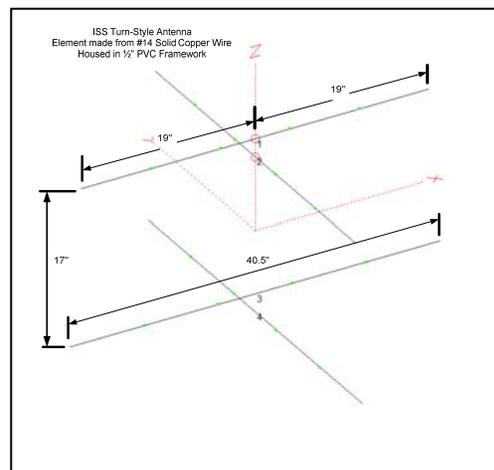
The actual antenna elements are made from common #14 electrical wire available at home improvement stores (insulated or non-insulated). The simple wires are not rigid enough to maintain their shape as an antenna; therefore, the antenna elements are inserted into an exoskeleton made of common ½ inch PVC pipe. The PVC exoskeleton is connected together with simple PVC fittings.
