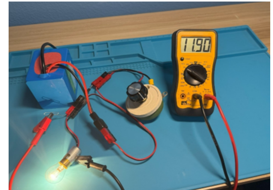
Rheostat set to full brightness. Diode inserted and forward biased, allowing current to flow. Light bulb voltage is 11.9 Volts.
