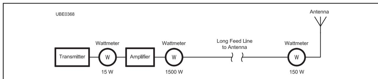
**Figure E-1** — This diagram shows a power level measured at the output of an Amateur Radio transmitter. The diagram also shows power levels after the signal goes through a power amplifier and a long length of coaxial cable.
