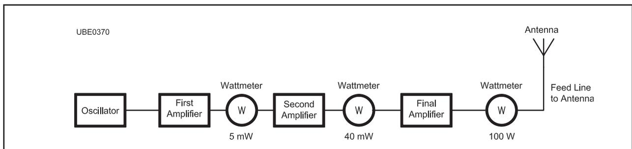
**Figure E-3 — A simple amateur transmitter amplifies the signal from an oscillator and then feeds that signal to an antenna. It uses several amplifier stages. The input power to one of those stages is 5 milliwatts and the output from that stage is 40 milliwatts. The text describes how to calculate the gain of that amplifier stage.**
