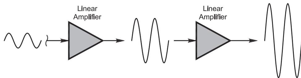
Each of these amplifiers has a gain of 3 decibels (3 dB). That means the output signal is twice as strong as the input signal.
