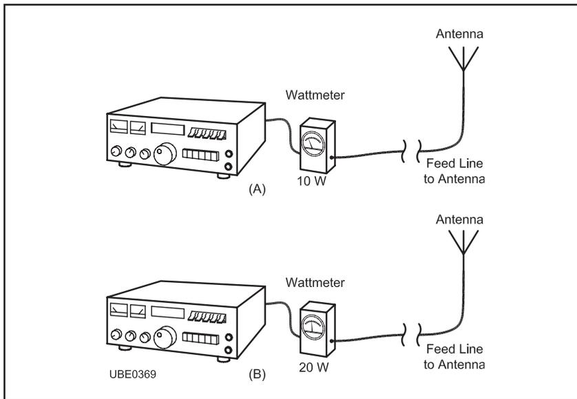
**Figure E-2 — The output power from an Amateur Radio transmitter is 10 watts. After making some adjustments to the transmitter tuning, you measure the power again. Now you find the power has increased to 20 watts. The text describes how to calculate the decibel increase that occurred.**
