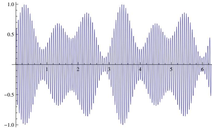
The AM signal after detection (demodulation, rectification):
