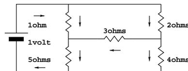
If the  $4\Omega$  resistor were  $10\Omega$ , then the impedance bridge would be balanced, there would be no voltage across the  $3\Omega$  resistor and no current through it.
