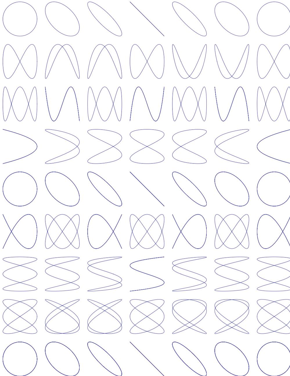
In this figure, the signals are sine waves. The phase varies from  $0^\circ$  in  $30^\circ$  increments to  $180^\circ$  horizontally. Vertically, there are three blocks of three rows of subfigures. In the subblocks, the horizontal base frequency is base frequency, second harmonic and third harmonic. Within each subblock, in each line of figures, the vertical input is base frequency, second harmonic and third harmonic.
