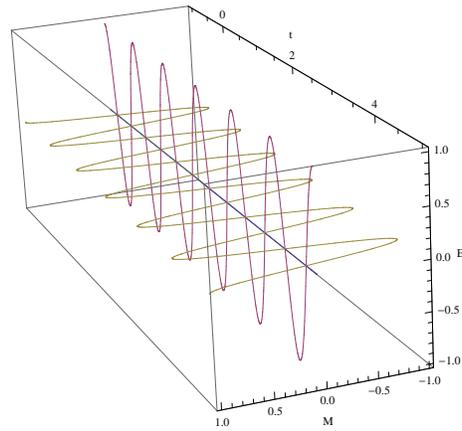
Left hand circularly polarized electromagnetic wave (one surface is the E field and the other is the M field):
