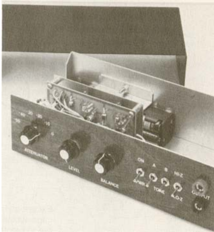
Exterior view of the two-tone audio generator.
