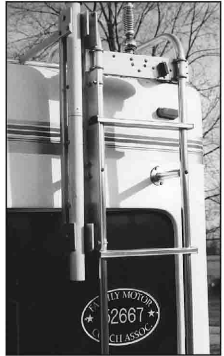
Figure 3—The author's manual tilt-over antenna mount. A removable pin locks the PVC antenna base into position, and a weatherproof switch selects the antenna in use.
