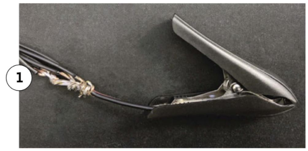
Combine the bare ends of the radial wires into a single wire, and solder them all together. To this connection, solder a single wire about 6 inches in length. This will attach to the ground side of your antenna system. To make the ground attachment, we soldered the single wire to a large alligator clip.
