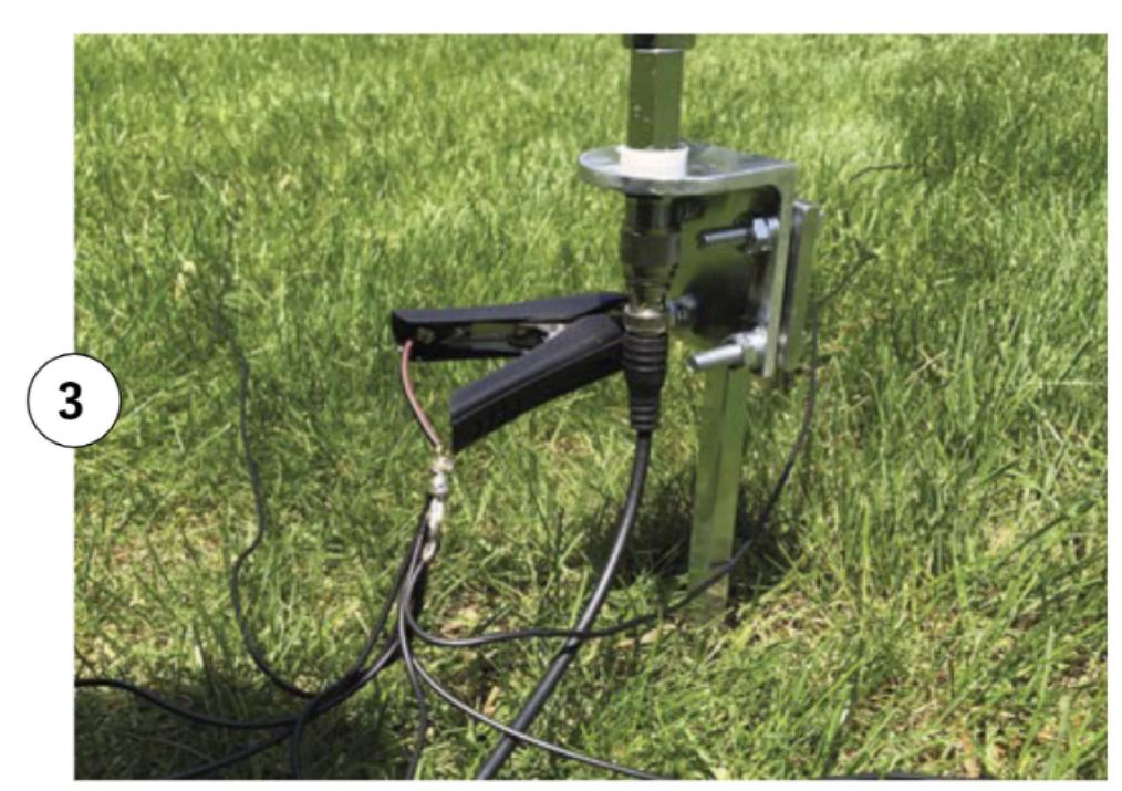
Take the antenna mount outdoors to your chosen spot, attach your coaxial cable to the mount, and then drive the support post into the ground. Attach the wire that connects to your six radials to the mount. In this example, we used a large alligator clip that simply attached to one of the mount's bolts.
