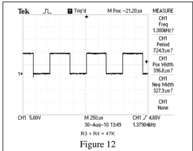
Plugging the values R1 = 10 K, R3 = 47 K, R4 = 0 (the variable resistor is set to 0 ohms), and C2 = .01 uF (or 1x10<sup>-8</sup>F) into the on-time formula, the result is 395.0 uS. [Remember the units must be in Ohms and Farads for the formulas to work]
