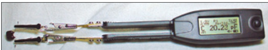
Figure 11 — The author's leaded component adapter.
