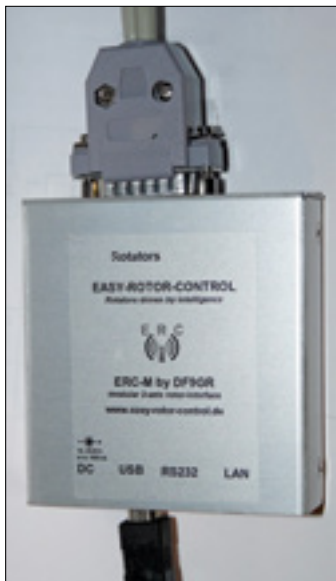
Figure 8 — The ERC-M rotator controller in its slimline case. A USB cable connects to the station computer, and both rotators are connected to a single 15-pin connector.
