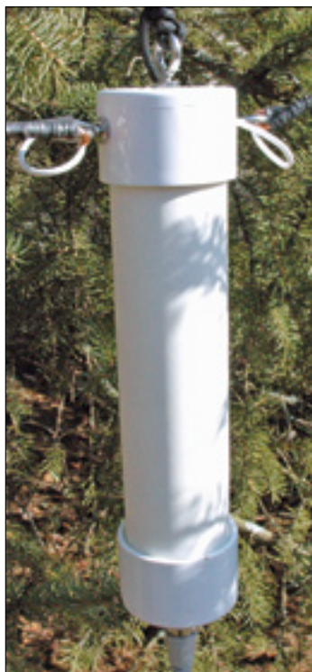
Figure 15 — The matching unit at 28 feet above ground.
