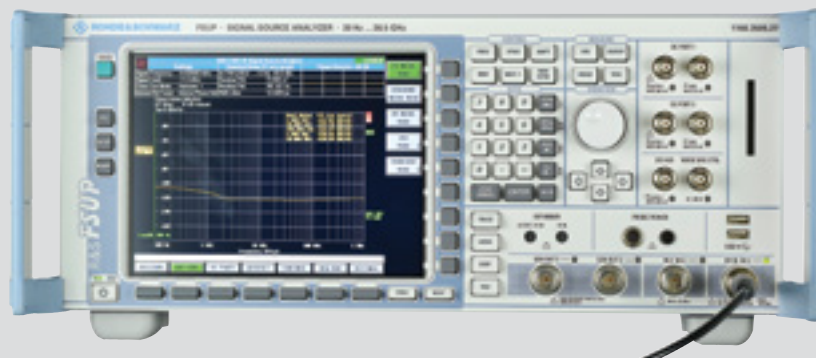
Figure A — The ARRL Lab's new Rohde & Schwartz FSUP 26 Signal Analyzer, used for transmitter phase noise testing.
