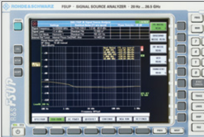
Figure B —The FSUP 26 screen shows quite a bit of detail during testing of the Hilberling PT-8000A on the 14 MHz band.
