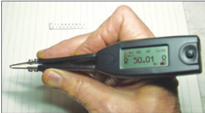
Figure 10 — The ST5 measuring a precision 0201 50 Ω SMD resistor.
