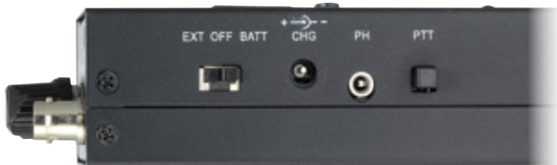
Figure 2 — The power switch, PTT switch, charging jack, and headphone jack are arranged along one side of the case.
