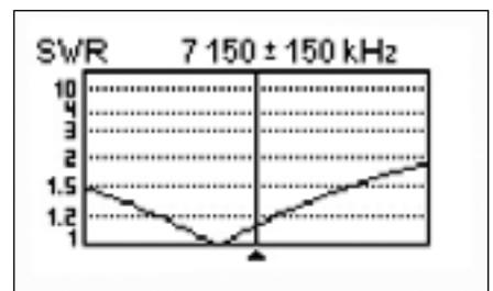
**Figure 4** — Measured SWR of the EFHW-8010 in the reviewer's station across 40 meters. Note that the full band is covered at less than a 2:1 SWR.
