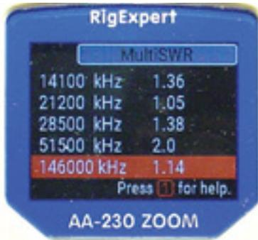
**Figure 8** — Using the AA-230 ZOOM's multi-band feature to check the author's TH1 antenna on 20,15,10, 6, and 2 meters.
