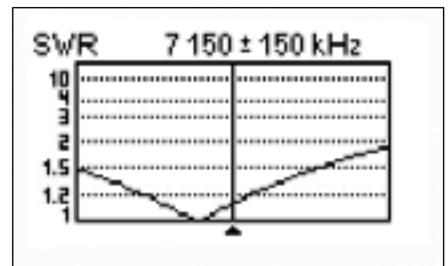
**Figure 4** — Measured SWR of the EFHW-8010 in the reviewer's station across 40 meters. Note that the full band is covered at less than a 2:1 SWR.
