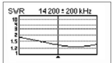
**Figure 3** — Measured SWR of the EFHW-8010-1K in the reviewer's station across 20 meters. This is fairly typical of what we observed.
