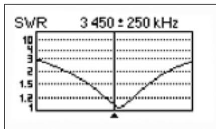
**Figure 7** — Measured SWR of the EFHW-8010 in the reviewer's station with the antenna analyzer centered below the bottom of 80 meters. This is indicative of how the antenna would operate over 80 meters if it were shortened to move its resonance to mid band.
