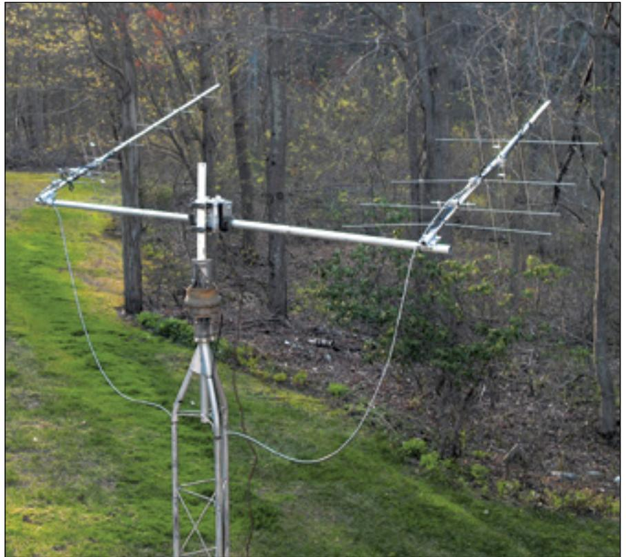
**Figure 1** — The 2 meter and 70 centimeter antennas installed on the crossboom and mounted on a short tower. (Note that the author accidentally bent one of the 2 meter reflectors slightly while installing the antennas. The elements were all perfectly straight when delivered.)
