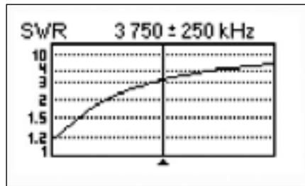
**Figure 6** — Measured SWR of the EFHW-8010 in the reviewer's station across 80 meters. Note the very low SWR at the bottom of the band. The manufacturer suggests trimming for best SWR. Based on a dipole model, removing about 8 feet of wire should bring it right in.
