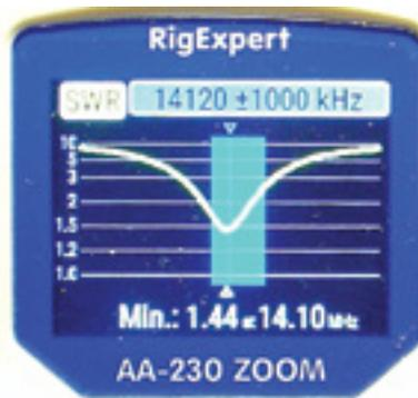
**Figure 11** — A direct 20 meter scan (not using the ZOOM feature).
