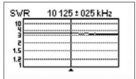
**Figure 5** — Measured SWR of the EFHW-8010 in the reviewer's station across 30 meters. This was the band with the worst SWR, and still likely within the range of "trimming" type antenna tuners.
