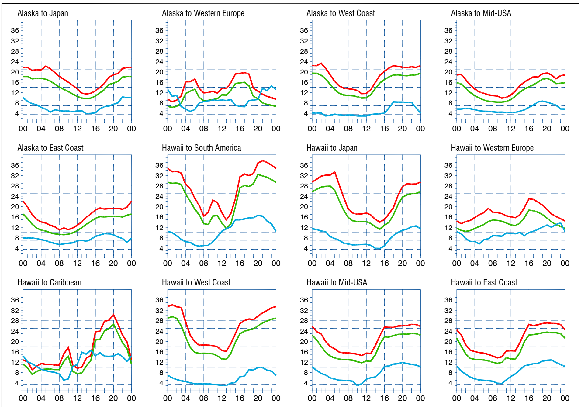
When are the bands open? These charts, generated using CAPman, show probabilities for average HF propagation in the month of September for the paths indicated. The horizontal axes show Coordinated Universal Time (UTC), and the vertical axes frequency in MHz. On 10% of the days of this period, the highest frequencies propagated will be at least as high as the upper red curves (HPF, highest possible frequency) and on 50% of the days they will be at least as high as the green curves (MUF, classical maximum usable frequency). The blue curves show the lowest usable frequency (LUF) for a 1500-W CW transmitter. For SSB or a lower transmitter power, the LUF will be somewhat higher than the blue curves indicate. See Oct 1994 QST , pp 27-30, and Feb 1995 QST , pp 34-36, for more details. The predictions assume an observed 2800-MHz solar flux value of 88. This is a Low level of solar activity. See the detailed propagation tables on The ARRL Antenna Book CD-ROM .
