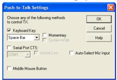
It's a bit confusing because this is not where you want to set the control of the rig for transmitting from a remote site. This screen applies to using your computer to access the link (where the actual receiver and transmitter are located), not the remote link. Leave it set with the defaults using the space bar. The Security tab is an important one.
