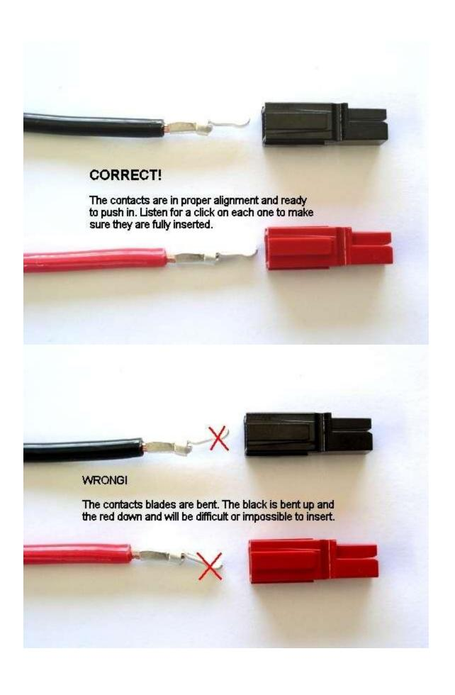
Tug slightly on the assembled connector to make sure the contacts are locked in place. If you have trouble getting the contact to lock in to the housing you may have squashed the contact wider deformed it some how. Look at the side profile of the contacts before and after crimping, you may have to bend it back straight before inserting it in to the housing.
