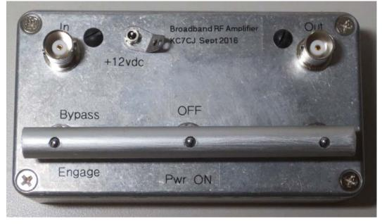
External view of completed amplifier with switch linking bar in place.
