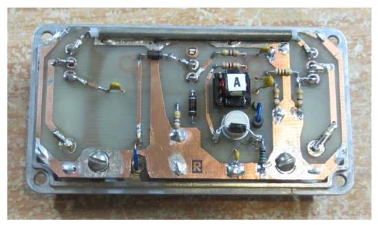
PCB assembly is mounted on enclosure lid. Diode CR2 and transistor Q1 are thermally bonded.
