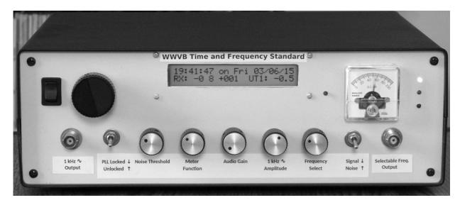
Figure 20 — Front view of the frequency standard in operation. The large knob on the upper left permits manual fine tuning of the VCTCXO, while the display provides the UTC date and time.
