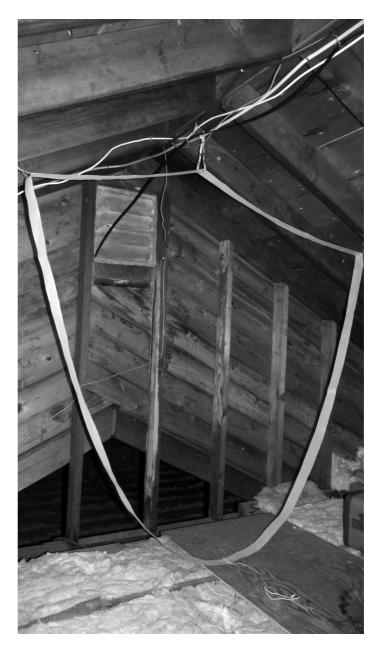
Figure 6 — The author's attic-mounted loop antenna. With the plane of the loop aligned toward Fort Collins, Colorado, the WWVB horizontally polarized H-Field cuts through the center of the loop and induces a voltage across it. The frequency standard amplifies and processes this signal.
