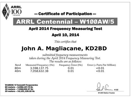
Figure 1 — The author's very successful Frequency Measuring Test results are achieved by using WWVB as a precision frequency reference.
