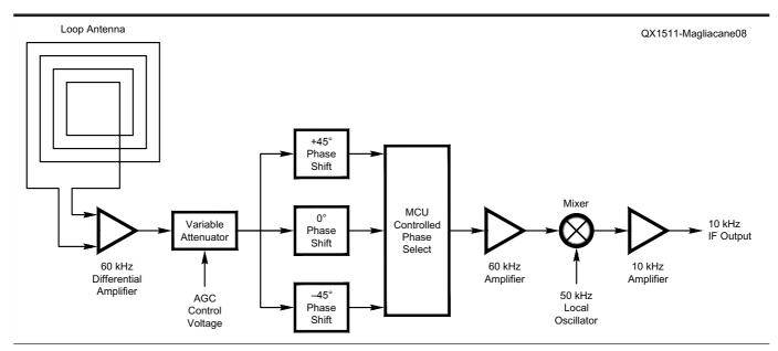
Figure 8 — This block diagram illustrates the overall RF to IF conversion process. The +45° and -45° phase shift networks were used in the past to compensate for the WWVB hourly phase signature, but have not been required since the introduction of BPSK modulation was made in 2012.
