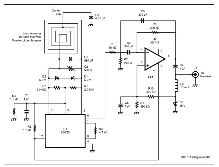
Figure 7 — 60 kHz WWVB loop antenna preamplifier. In addition to providing 40 dB of gain, the preamp properly interfaces the balanced loop antenna with the ground-referenced circuitry in the frequency standard.
