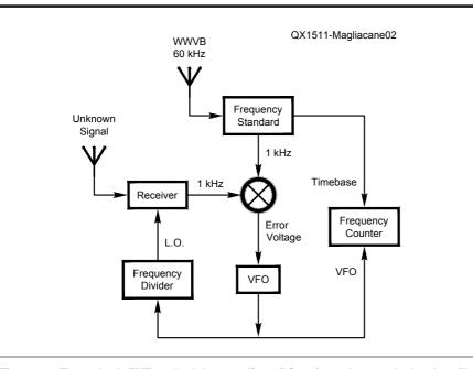
Figure 2 — The author's FMT methodology applies a DC tuning voltage to the local oscillator of a direct conversion receiver to lock its audio output in phase with that of a 1 kHz reference. The frequency of the unknown signal is determined by measuring the frequency of the LO and factoring in the 1 kHz tuning offset.
