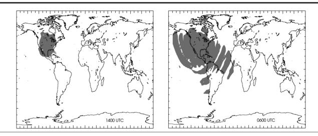
Figure 3 — Space and Naval Warfare Systems (SPAWAR) Command computer simulations illustrate how the WWVB 100 μV/m signal level contours contract during the day and expand during nighttime hours. (Images from NIST website.)
