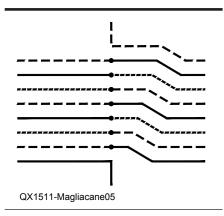
Figure 5 — Loop antenna construction. The ends of the multi-conductor cable are brought together at the bottom of the loop to form a multi-turn coil. After going around once, the end of conductor #1 connects to the beginning of conductor #2, conductor #2 connects to conductor #3, and so on.
