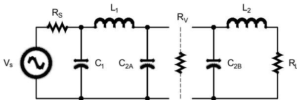
Figure 7 — Here, the pi-L network is divided into a pi network followed by an L network. The resistance looking into the input of the L network is  $R_V$ ; this is also the load resistance for the pi network.
