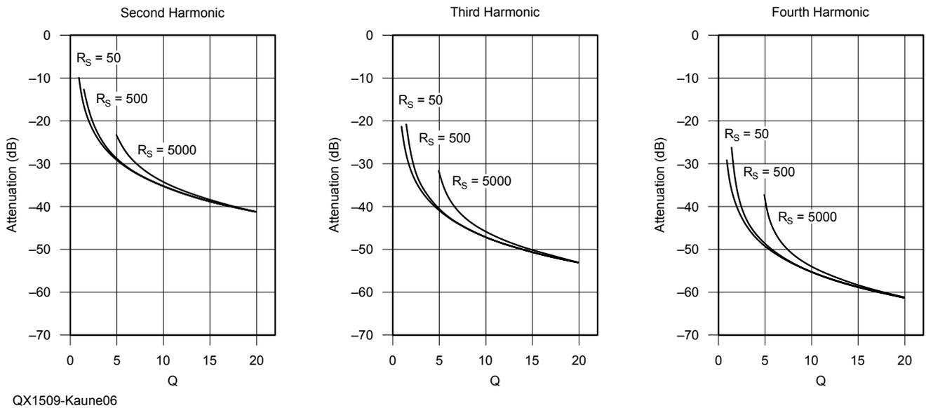
Figure 6 — These graphs plot the attenuation of second, third and fourth harmonics by a pi network as a function of  $Q$ . Data are shown for load resistance of  $50\ \Omega$  and source resistances,  $R_S$ , of 50, 500, and 5000  $\Omega$ .
