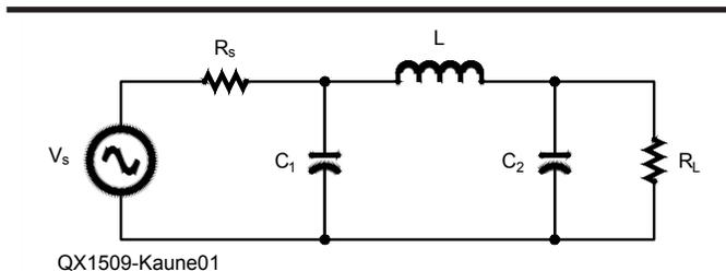
Figure 1 — This schematic diagram shows a low-pass pi network.
