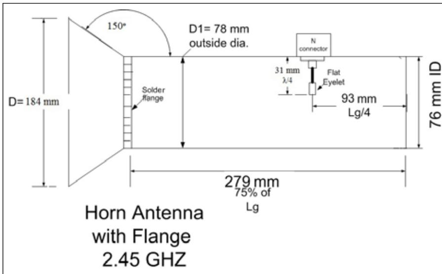
Figure 17 – Diagram of Complete Hooded Horn antenna.
