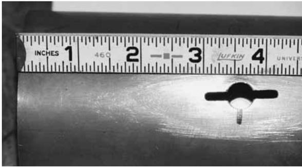
**Figure 7 — Drilled opening for type “N” connector probe assembly. The slot was tried to be able to move the probe for best results. No difference was found and the slot was eliminated on later models.**
