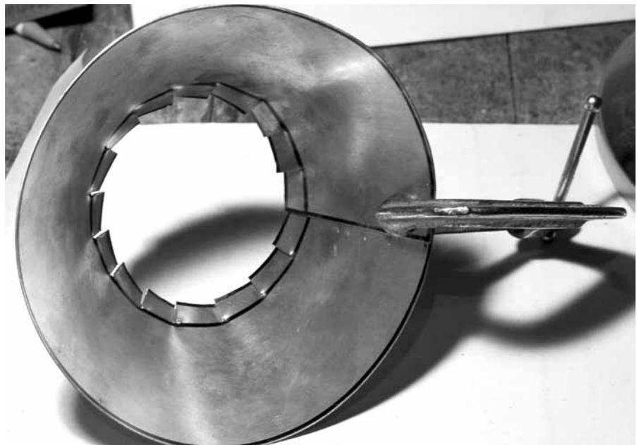
**Figure 15 — Bend the flange into a circle, holding with vise grips, solder the seam.**
