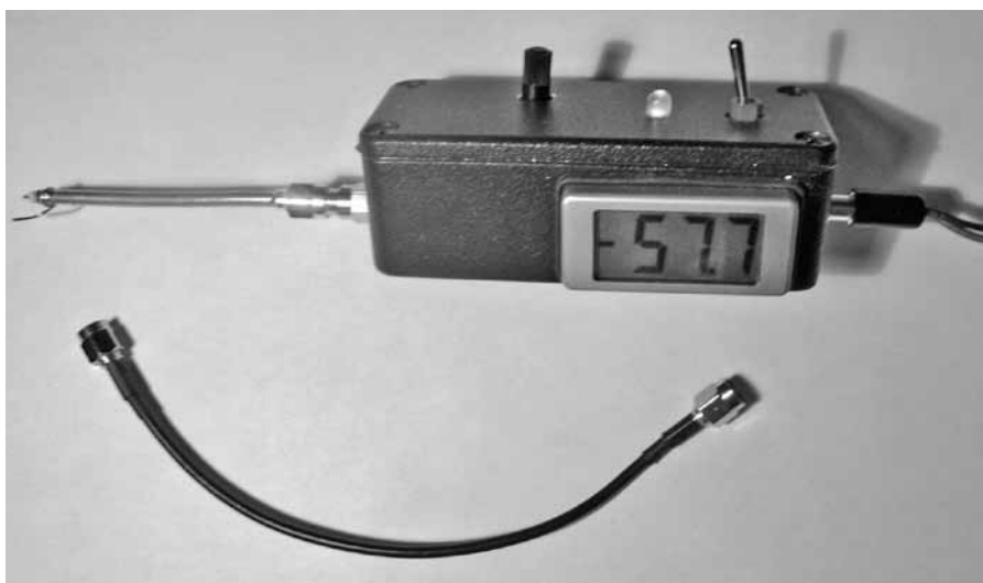
Figure 1 — The finished assembled power meter.
