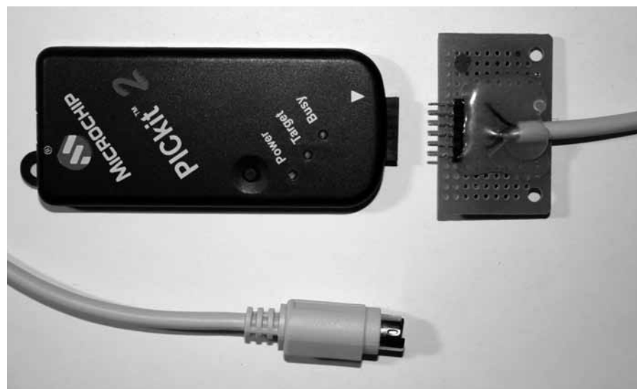
Figure 5 — This photo shows a PICkit 2 programming cable wired using the connections shown in Table 2. Hot glue protects the cable connections to a small prototyping board. The dark colored dot on the top left corner of the perf board is oriented with the white triangle on the PICkit 2.
