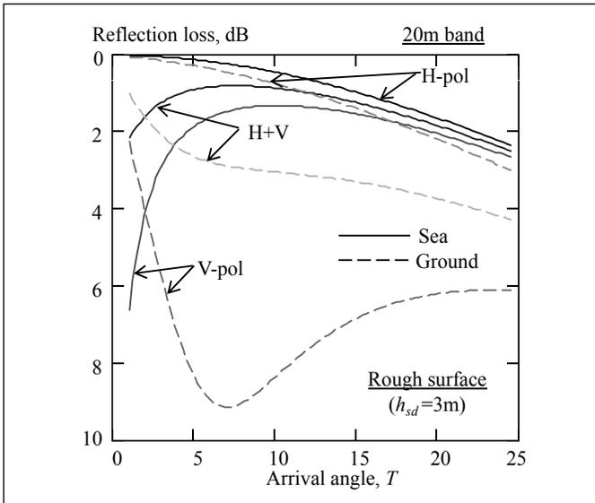
**Figure 4 — Reflection coefficient with surface roughness, 20 m band.**
