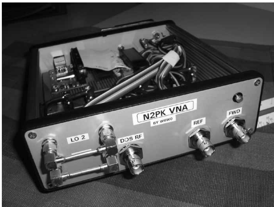
Figure 1 – The N2PK dual-detector VNA.
