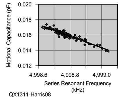
Figure 8 — Here is a plot of the motional capacitance,  $C_m$ , versus series resonant frequency,  $f_s$ , for the batch of crystals.
