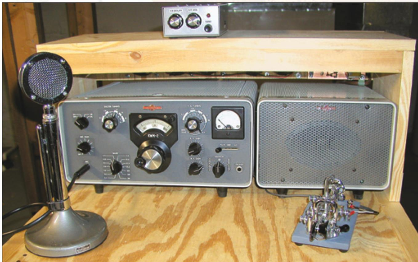
as information for those who may wish to improve KWM-2 CW operating performance by means of BFO carrier shift. The intent is to generate true carrier CW operation and bring the received tone to 800 Hz while copying CW. These modifications do not change SSB operation of the KWM-2 transceiver. All circuit changes are reversible if it is desired to return the transceiver to its original state.
