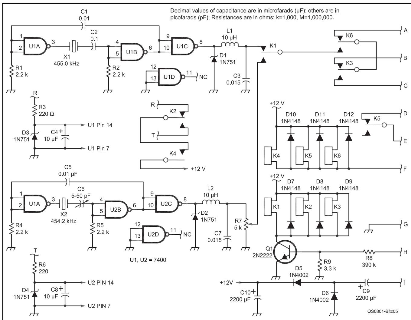
Figure 5 — Schematic diagram and parts list for new KWM-2 BFO board.
