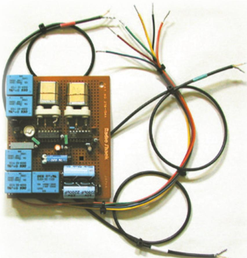
Figure 6 — Photo of the new KWM-2 BFO board.
