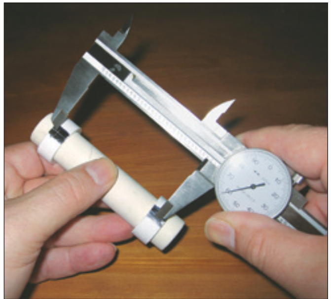
Figure 11 — Using dial caliper to accurately mark dimension E.
