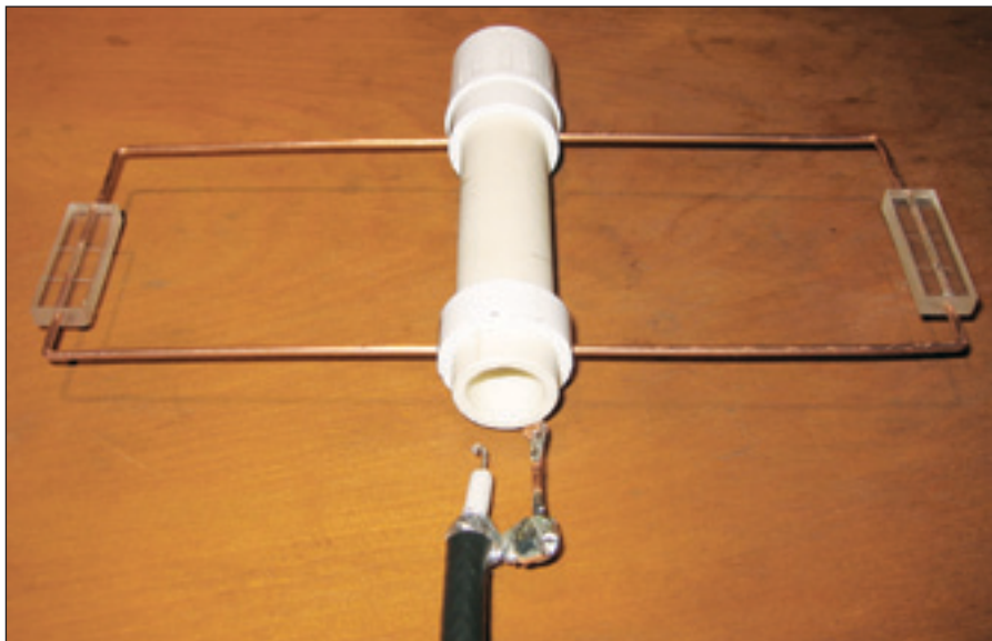
Figure 12 — Core with driven element (bottom) and reflector prior to attaching feed line.
