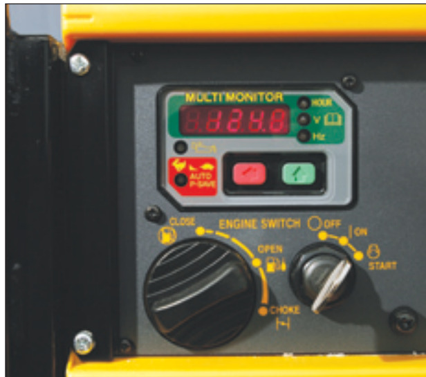
Figure 5 — Inverter generators, a bit larger than the relatively small units examined in the article, often feature voltage, frequency and run-time monitors. You'll know when to change the oil — and you'll have peace of mind when powering your sensitive gear.
