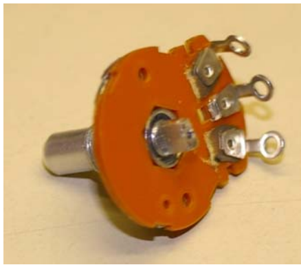
Figure 5: Potentiometer ready for photodiode and chopper.
