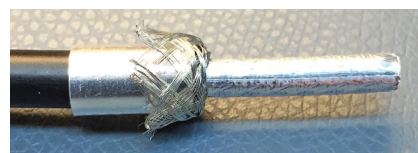
Figure 4 — The cable braid shown trimmed and folded back.
