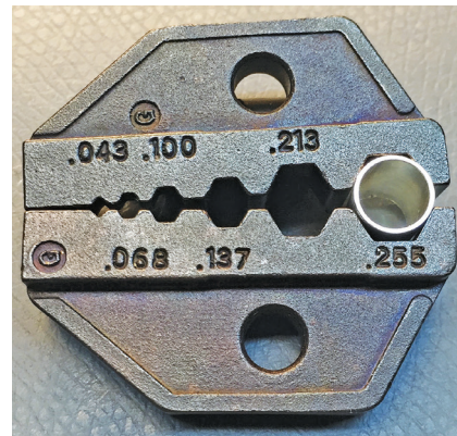
Figure 8 — An unmounted die, illustrating proper placement of ferrule for crimping.
