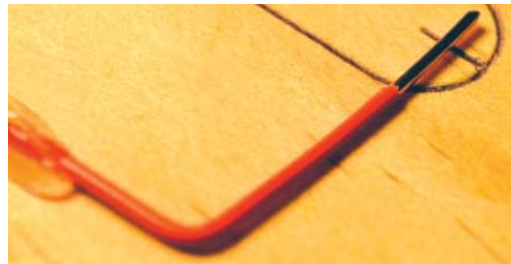
Figure 4 — The long section of the wire is glued to the wood, alongside the traced outline of the craft stick.
