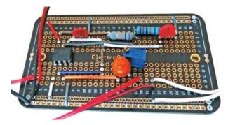
**Figure 2** — The ElectroCookie breadboard with the parts mounted. Try to copy this layout exactly to avoid errors, though a socket for the NE555 timer chip is optional. Schematic designator R3 adjusts the volume; the lower the volume, the less current the circuit draws.
