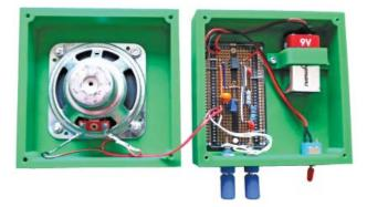
**Figure 3** — The 3D-printed CPO housing consists of a base that accommodates the PCB, the battery with a clamp, the power switch, and banana receptacles for the keyer. The cover houses the speaker.
