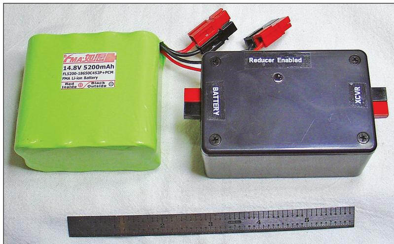
**Figure 5** — The assembled voltage reducer alongside a four-cell 5200 mAh LiPo battery. Even though the battery label lists 14.8 V, a freshly charged four-cell LiPo battery will have a voltage of 16.8 V, which is too high for most portable radios.
