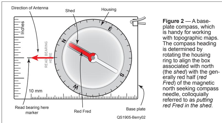
**Figure 2** — A baseplate compass, which is handy for working with topographic maps. The compass heading is determined by rotating the housing ring to align the box associated with north (the *shed*) with the generally red half (*red Fred*) of the magnetic north seeking compass needle, colloquially referred to as *putting red Fred in the shed*.
