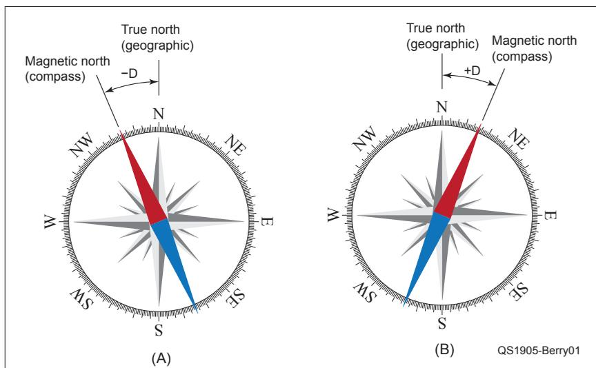
**Figure 1** — At (A), the absolute value of a westward declination must be added to the heading shown by the needle (colloquially known as *red Fred*) to determine true north; at (B) for an eastward declination, the declination is subtracted from the magnetic heading to determine true north.
