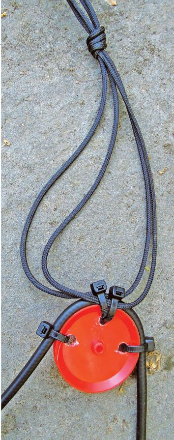
Coax cable strain relief plastic pulley assembly.
